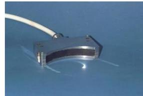
**Curved Probe for Electronic scanning of weld area**
